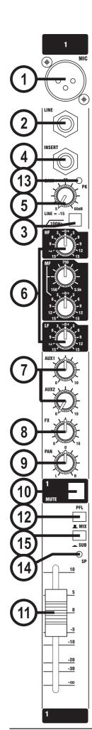
The Send may also be tapped off as an alternative pre-fade, pre-EQ direct output if required, using a lead with tip and ring shorted together so that the signal path is not interrupted (see below).
